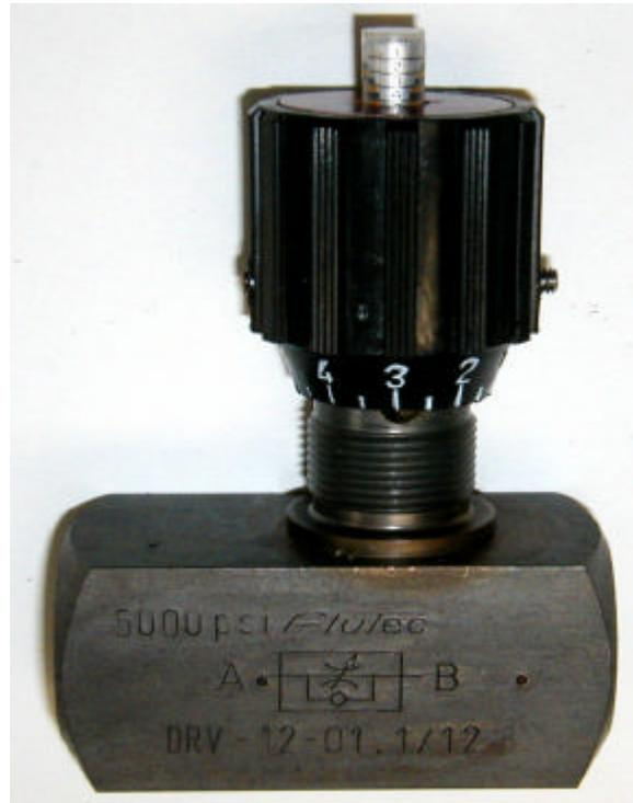
To turn the Knob and adjust the valve, loosen a set screw with a 5/64 inch hex key wrench, this will allow the knob to be rotated. Turn the knob till the indicator extends to its maximum as shown in the photo (above). Tighten the set screw to prevent the valve from closing.
