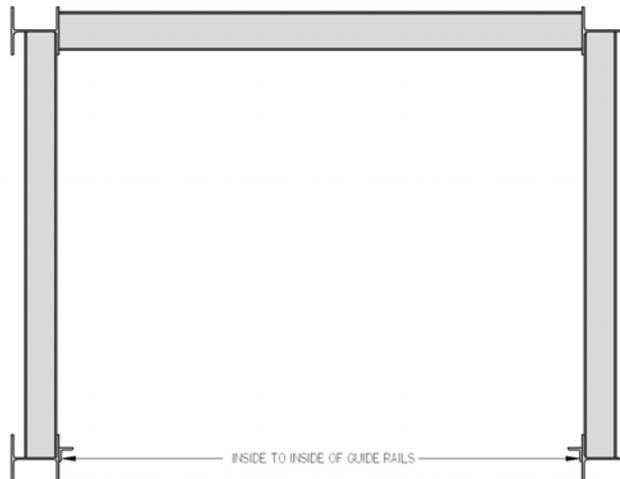
2. Measure the outside to outside distance of the guide runners on the top drive. For proper adjustment side to side of the top drive in the mast there should be 1/8" to 3/16" gap between the guide runners on the top drive and the narrowest point in the mast.
