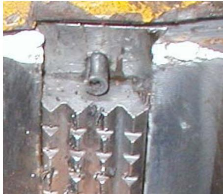
2. Perform daily inspection of retainer pins to ensure they are in place and not damaged. Also inspect after suspected movement of assemblies without fully opened or closed gripper.
