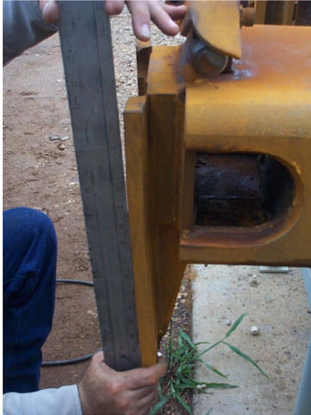
Figure 2: Bent Bottom Plate
