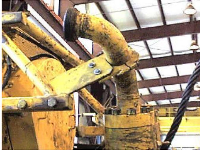
**Figure 5-Insufficient Support**
