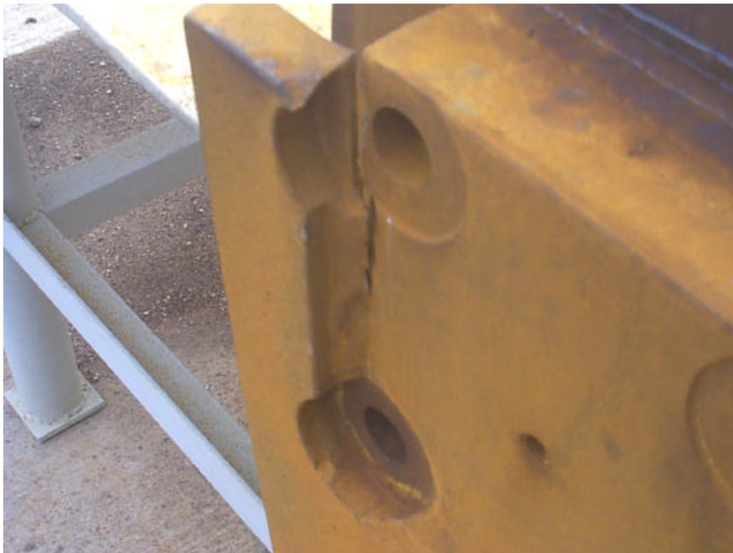
Figure 1: Typical Crack in a Slide
