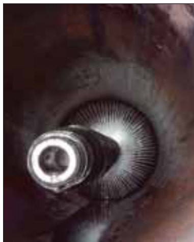
1.69 in. OD Retrievable Bridge Plug set in 7 in. 26.00 lb/ft (6.276 in. ID) Casing
