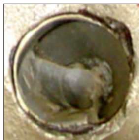
DL—Stinger element delamination.
