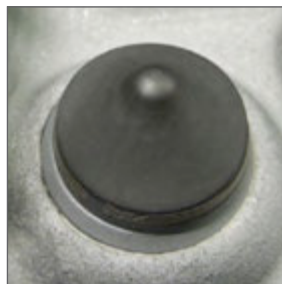
WT—No wear (Level 0 severity).
