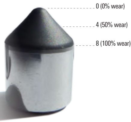
WT—No wear (Level 0 severity).
