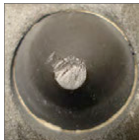
WT—Minimal wear (Level 1 severity).
