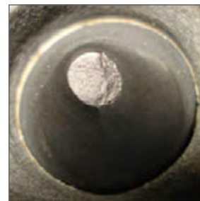
WT—Minor wear (Level 2 severity).
